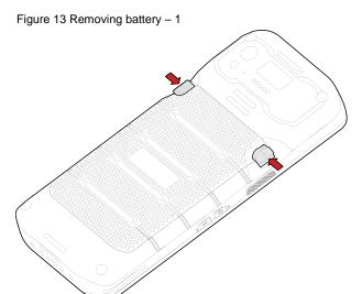
2. While pressing the battery release buttons in, pull the battery up.
