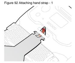
2. Insert the arrowhead into the small hole of the hand strap and pass it through the neck.
