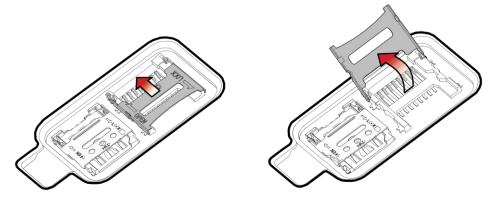
3. Put the SD card you prepared with the contacts facing down.
